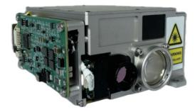
LDR60K1 1064nm Laser Rangefinder & Laser Irradiation. The ranging capability for NATO targets is  $\geq$  12 km. The ranging frequency is 1~ 20 Hz. The laser illumination distance is  $\geq$ 6 km. The pulse width is  $\geq$  15 ns  $\pm$  5 ns. The beam divergence angle is  $\leq$  0.30 mrad. The weight is  $\leq$ 680 g.
