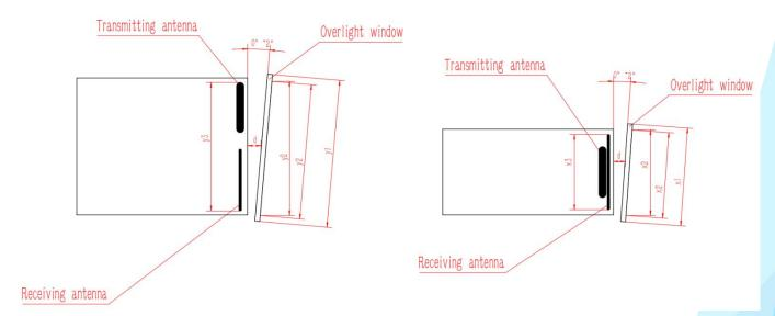
The effective aperture of the optical window  $y_2$  - the outer diameter of the optical window  $y_1{>}2mm$
