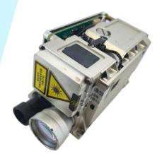
LDR40K1 1064nm Laser Rangefinder & Laser Irradiation. The ranging capability for NATO targets is  $\geq$  6 km. The ranging frequency is  $1\sim20$  Hz. The laser illumination distance is  $\geq4$  km. The pulse width is  $\geq15$  ns  $\pm$  5 ns. The beam divergence angle is  $\leq0.4$  mrad. The weight is  $\leq460$  g.
