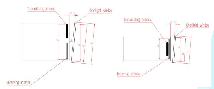
The effective aperture of the optical window  $y_2$  - the outer diameter of the optical window  $y_1\!\!>\!\!2mm$
