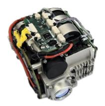
LDR25K1 1064nm Laser Rangefinder & Laser Irradiation. The ranging capability for NATO targets is  $\geq$  5 km. The ranging frequency is  $1\sim20$  Hz. The laser illumination distance is  $\geq2$  km. The pulse width is  $\geq15$  ns  $\pm$  5 ns. The beam divergence angle is  $\leq0.6$  mrad. The weight is  $\leq380$  g.
