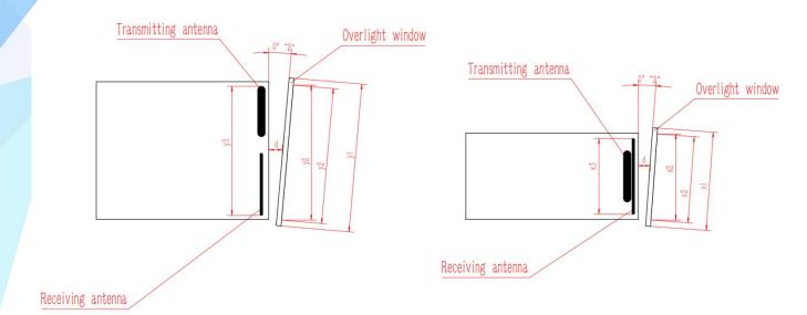
The effective aperture of the optical window  $y_2$  - the outer diameter of the optical window  $y_1>2mm$
