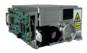
LDR80K1 1064nm Laser Rangefinder & Laser Irradiation. The ranging capability for NATO targets is  $\geq$  16 km. The ranging frequency is  $1\sim20$  Hz. The laser illumination distance is  $\geq8$  km. The pulse width is  $\geq15$  ns  $\pm5$  ns. The beam divergence angle is  $\leq0.30$  mrad. The weight is  $\leq680$  g.
