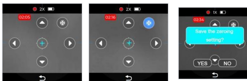
Figure 11 — Zeroing screen, correction keys and save prompt
