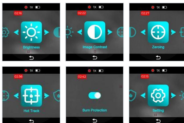
Figure 10 — Menu icons: brightness, contrast, zeroing, hotspot tracking, bright-light protection and settings
