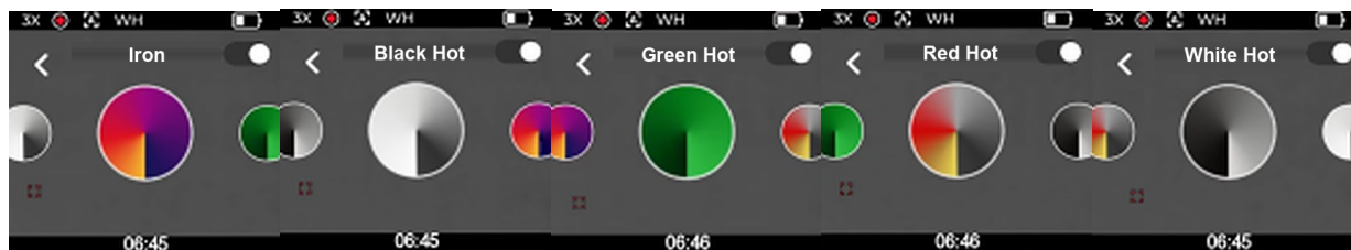
Figure 8-3 Image palettes: iron, black hot, green hot, red hot, white hot
