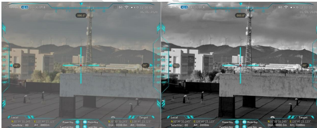
Figure 25 Fog-penetration effect in TV mode (left: fog penetration off; right: fog penetration on)
