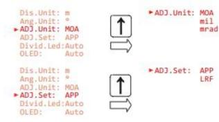
Sets the unit of the ballistic solution correction.
