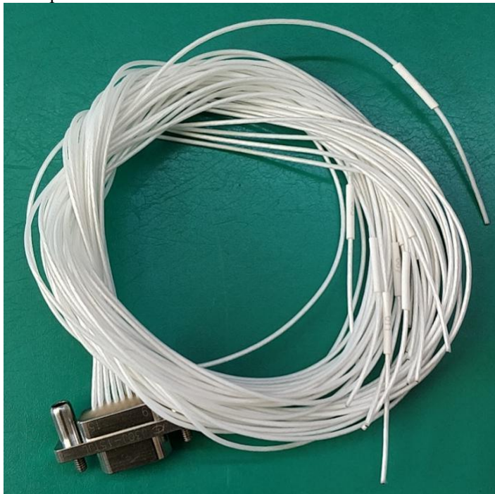
Figure 3 Host computer cable
