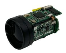
LRF1200A2 laser ranging module is a new lightweight and compact ranging module, operating at a wavelength of 905nm. The maximum range of the product is ≥1200m, using a UART-TTL interface and supporting test software, which is convenient for users to further develop. It has the characteristics of small size, light weight and reliable performance. It can be used in aviation, communications, geology, police, outdoor sports and other occasions.
