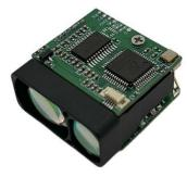
The LRF1500A laser distance measurement module is a new type of lightweight and compact distance measurement module operating at a wavelength of 905nm. With a maximum measuring range of  $\geq$ 1500m, it adopts the UART-TTL interface and is equipped with testing software, which facilitates further development by users. It features small size, light weight, and reliable performance. It can be used in aviation, communication, geology, policing, outdoor sports, and other occasions.
